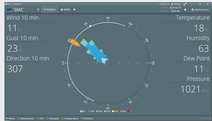
SMC Helideck Operation System for Yachts is a pre-configured and easy to install system to comply with Large Yachts and other vessels that have a Helideck. The system provides vessel motion and weather monitoring on one single SMC Panel Display
